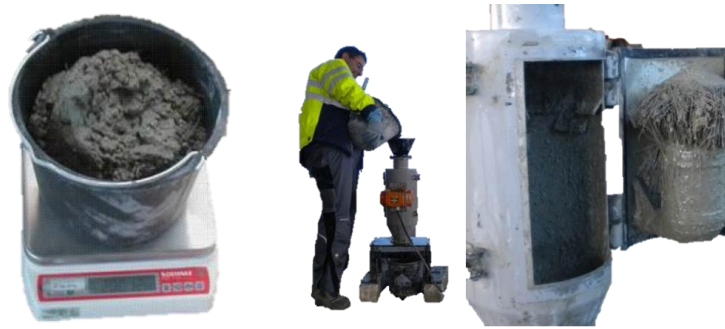
Figure 9. Wash-out test using pipe magnet.
