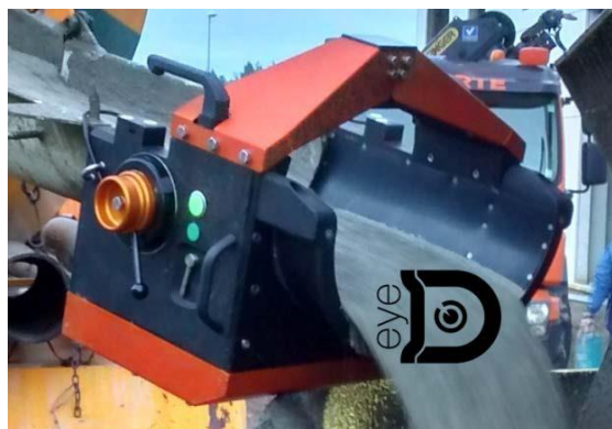
Figure 10. eyeD ® system connected to the chute of a truck mixer.
