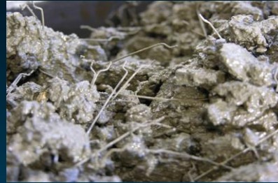
More efficient and easy to use steel fiber reinforced concrete
