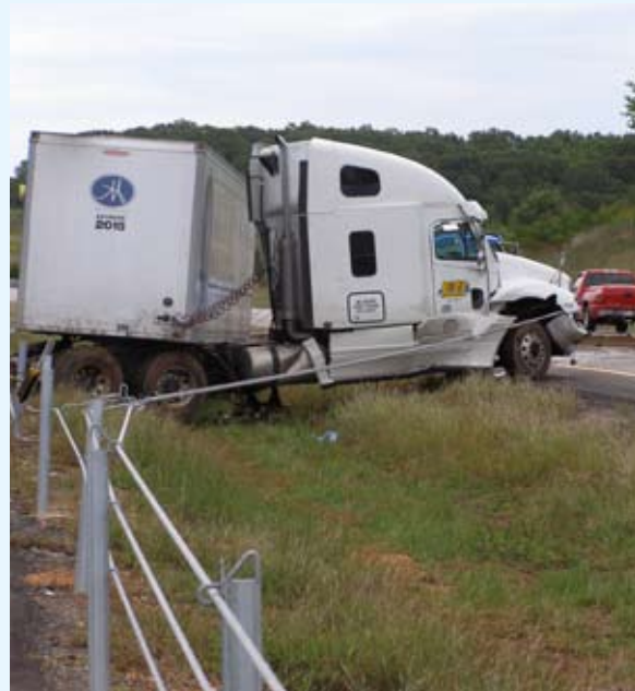
Bekaert and Gibraltar cooperated on a cable barrier that received a K-12 rating. The barrier can stop an LB truck weighing 15 000 lb colliding head-on at 80 km per hour.
