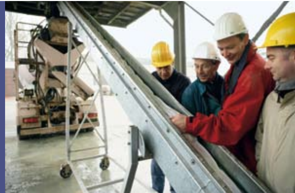
The Dramix® Booster adds automatically the right quantity of Dramix® steel fibers to the concrete mix.
