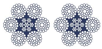
Non Dyform wire rope on adjacent drum laps can cause point contact and accelerated wear.
