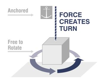
The torque or turn generated will increase as the load applied increases. The degree to which a wire rope generates torque or turn will be influenced by the construction of the rope. Having recognised what can happen when a rope is loaded it is necessary to select the correct type of rope. It should be noted that all ropes will rotate to some degree when loaded.
