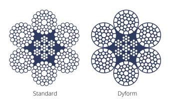
The smooth surface of the "Dyform" product provides improved rope to sheave contact leading to reduced wear on both rope and sheave . Increased cross-sectional steel area and improved inter - wire contact ensures that the rope will operate with lower internal stress levels resulting in longer bending fatigue life and lower costs.
