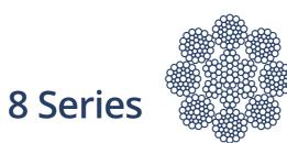
The 8 Series is a range of general purpose 8 stranded galvanized ropes produced with a steel core, fully lubricated during manufacture producing in accordance with EN 12385.
