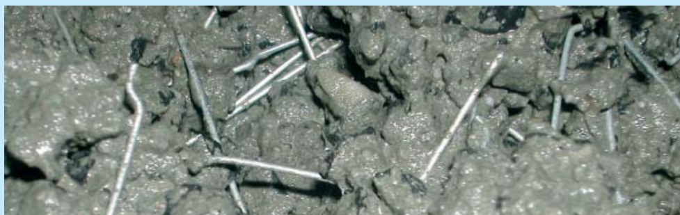
Dramix ® steel fibres make concrete stronger and prevent it cracking.
