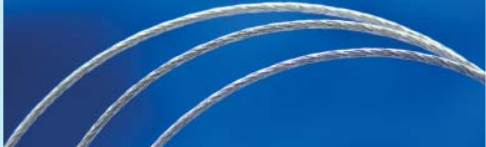
Impregnated fine cord is used to produce high-precision toothed polyurethane belts with superior corrosion resistance.
