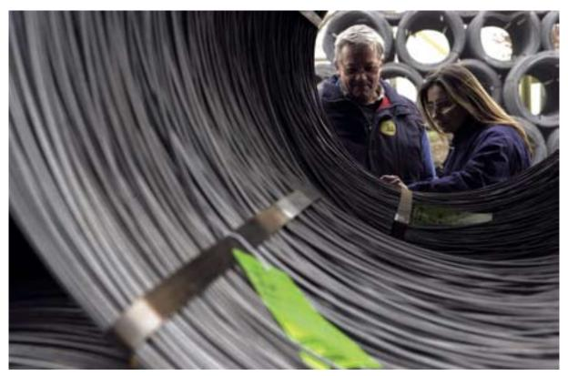
Wire rod is Bekaert's most important raw material. Bekaert buys wire rod in many different qualities and compositions to meet the most diverse production specifications.
