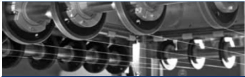
Figure 2 : Bekaert sawing wire is used in Meyer Burger solar wire-cutting machines
