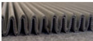
Bekaert Bekipor® ST: a nonwoven sintered porous structure.
