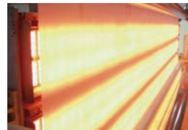
APP Gold East Paper - China Art Paper Bekaert GemDryer® Gem 10 1,800 m/min 16.5 MW 9.8 m
