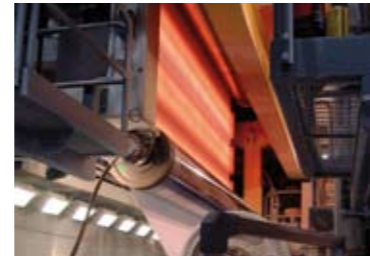
M-real Kajo - Finland Double Coated Fine Paper Bekaert GemDryer® Gem 9 1,200 m/min 8.2 MW 5.8 m
