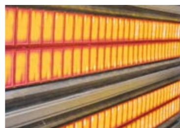
Cordenons Malmedy - Belgium Fine and Specialty Paper Bekaert UniDryer® V2 Gem 9 400 m/min 745 kW 3.1 m
