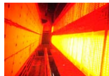
UPM Nordland Papier - Germany Coated Fine Paper Bekaert WebMate® M2000+Corad 1,600 m/min 36 MW 9.6 m
