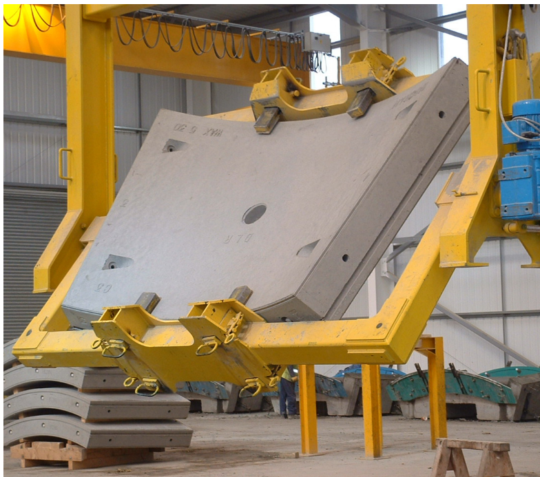
Segments casted in static moulds almost no damage in handling
