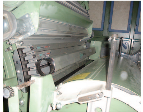
Trützschler DK760 equipped with XLXE6V stationary flats system results in improved yarn quality (lower IPI).
