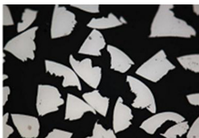
Cross-section of Bekipor® ST sandless spinpack
