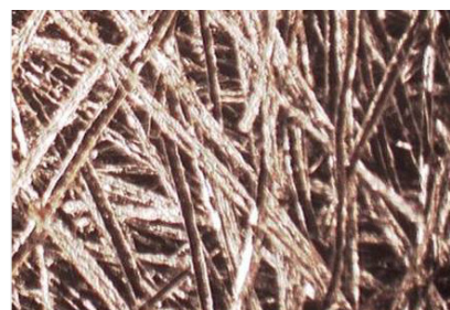
Top view of Bekipor® ST sandless spinpack
