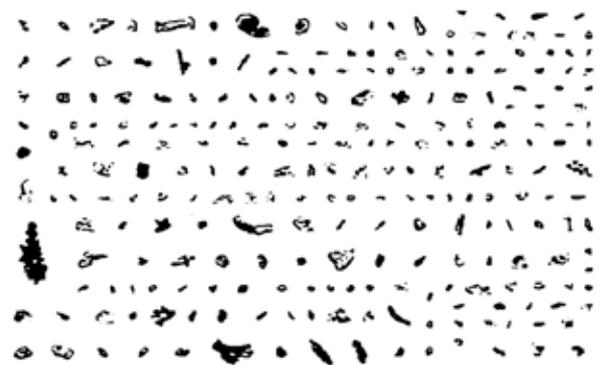
This is a close-up of particulate material in hydraulic fluid from a glass fiber filter. The smallest particle is 20µm while aircraft hydraulic systems require absolute filter ratings of 5µm.
