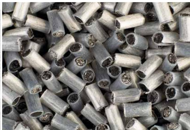
Grains of stainless steel fiber filler material
