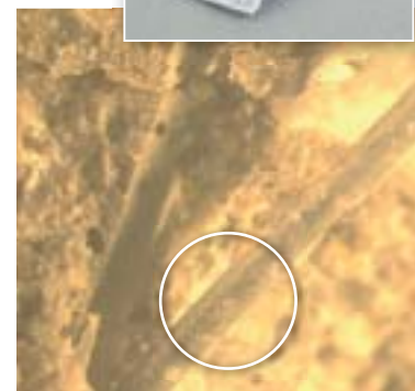
Smooth surface around Dramix® Green fibres with inhibitor
