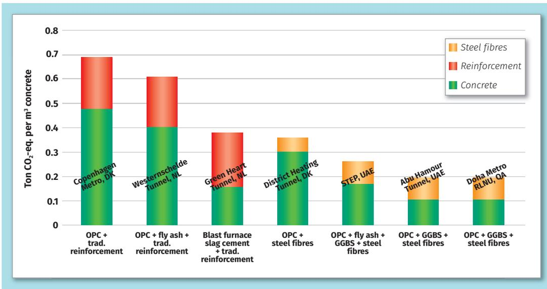
Left, figure 5: Comparison of embodied CO<sub>2</sub> for different types of binder and steel reinforcement used for major infrastructure projects (Edvardsen et al)
