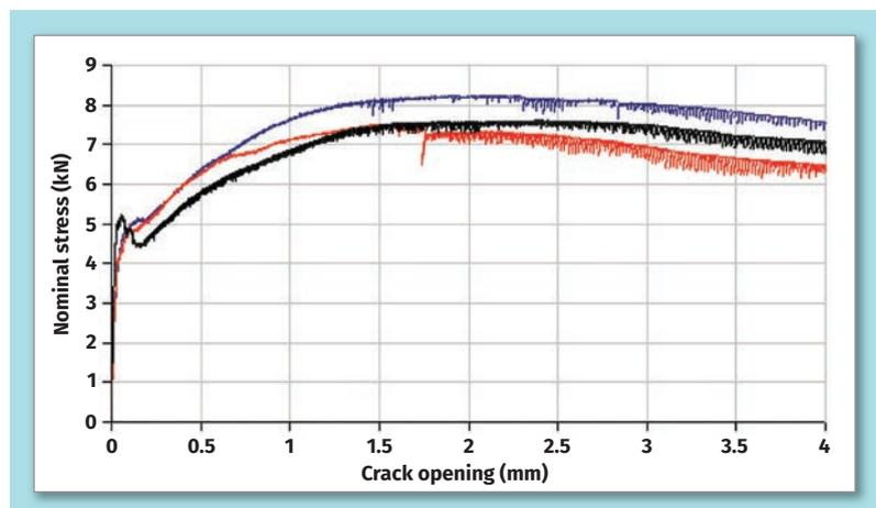
Above, figure 2: Typical results of beam tests of FRC according to EN14651 using 40kg/m<sup>3</sup> Dramix 4D80/60B
