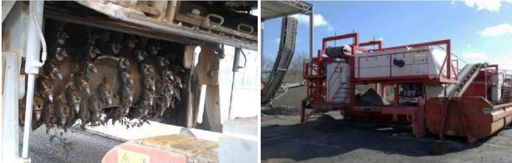
Figure 4: Left: Milling drum after grinding 100 m<sup>2</sup> asphalt reinforced with new steel grid. Right: Traditional breaking installation for asphalt foreseen with magnets.
