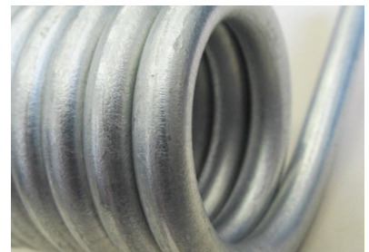
Excellent coating adhesion: wrap test on a 6 mm wire
