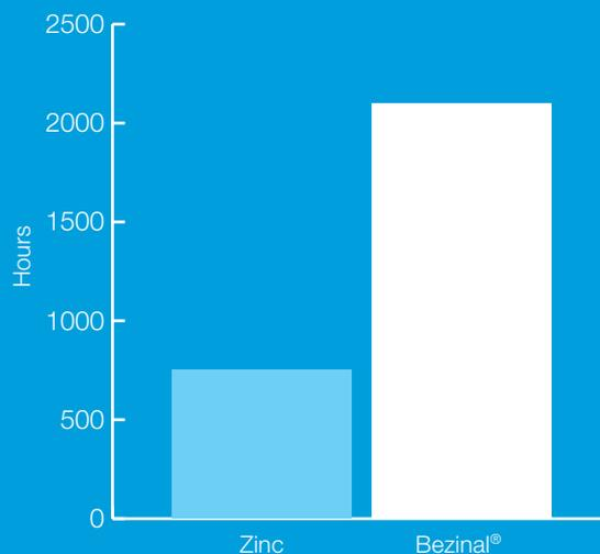
COATED SPRING AFTER SALT SPRAY TEST
