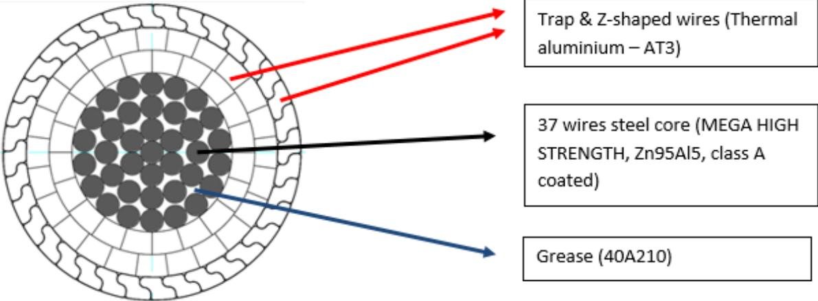
The core is composed by 37 steel wires, 3,38 mm diameter. The steel wires are protected against corrosion by a Zn95Al5 alloy coating (see paragraph 2.1.3 for details concerning steel grade and advantages of this type of coating).
