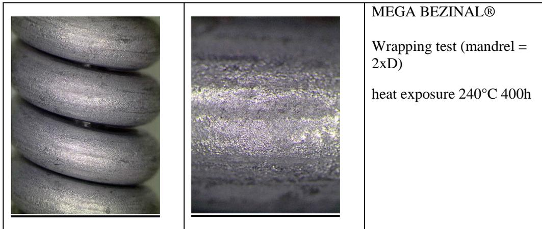
Additional heat exposure trials have been conducted to evaluate the impact on mechanical properties and coating adherence on these new steel grades. Bekaert compared different grades, ST4A, UHS, MEGA as such (not aged) and exposed to 240°C for 400 hours and 350°C for 24 hours.
