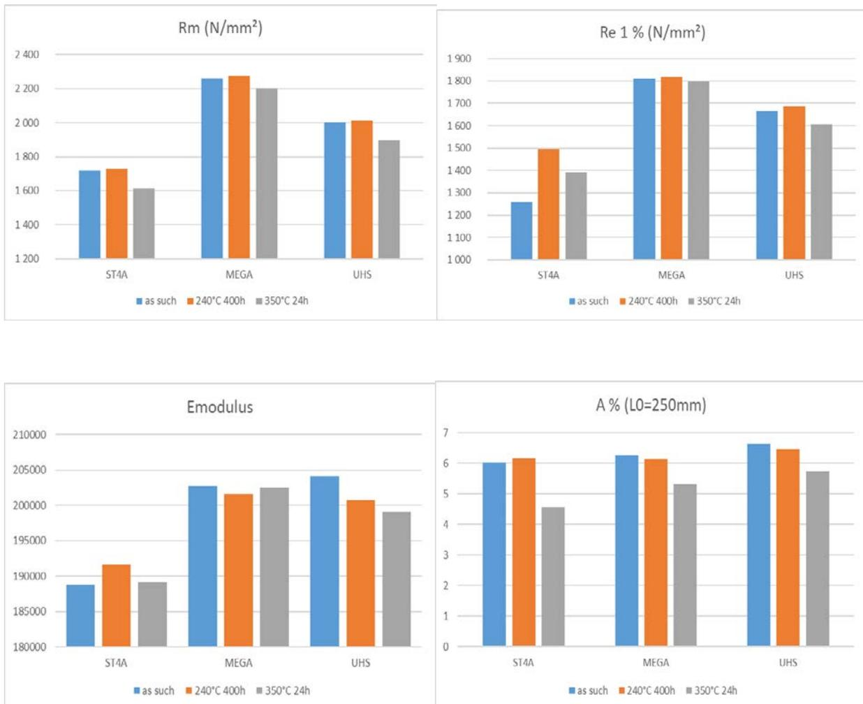
As conclusion, the behavior of the high tensile grades was comparable with current standard grades and showed a satisfactory stability after the different heat exposure conditions.
