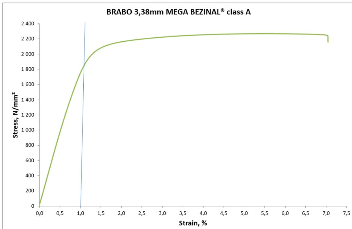
The steel composition used is a high carbon Chromium Vanadium micro-alloy on which an additional heat treatment has been applied in order to obtain the desired mechanical properties. Bekaert has extensive experience with this steel composition mainly in the offshore industry where the same steel grade is used for mooring lines for oil production platforms.
