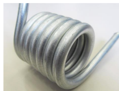
Wrapping test: 6mm Bezinox ® wire wrapped on a 18mm mandrel
