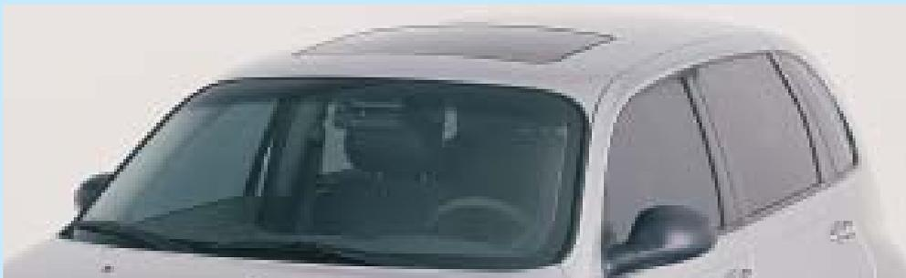
*As well as wire, Bekaert also supplies solar control and protective film for the automotive industry. In vehicles this film helps create a more pleasant in-car environment by improving temperature control, reducing reflections and shielding against harmful UV radiation.*
