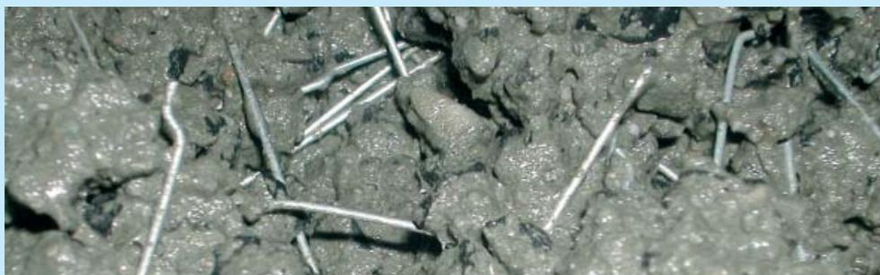
*Dramix*<sup>®</sup> steel fibres make concrete stronger and prevent it cracking.
