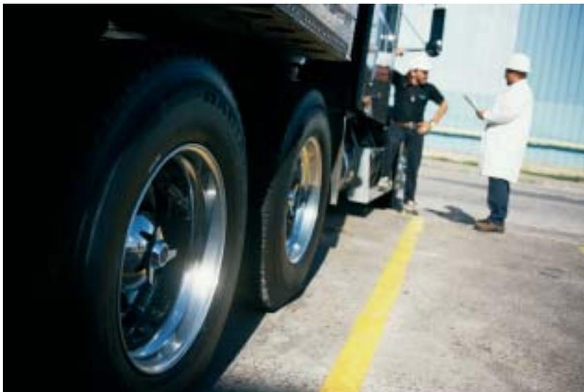
Each truck tire contains over 10 kg of ultrahigh-tensile steel cord. As well supporting the weight of the vehicle, steel cord reinforcement also helps to transmit steering, driving and braking forces to the road.
