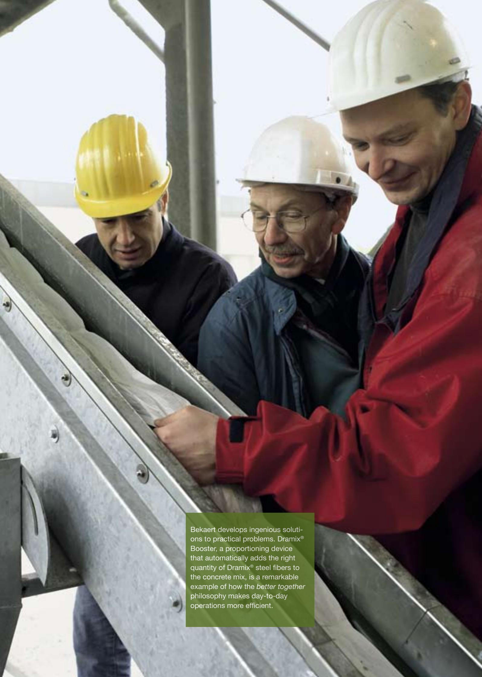
Bekaert develops ingenious solutions to practical problems. Dramix® Booster, a proportioning device that automatically adds the right quantity of Dramix® steel fibers to the concrete mix, is a remarkable example of how the *better together* philosophy makes day-to-day operations more efficient.
