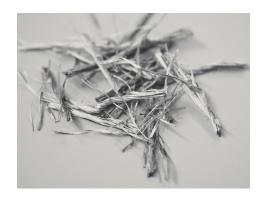
Synmix® EZ54 synthetic fibers are manufactured from 100% virgin polypropylene embossed monofilaments, twisted to a rope. Synmix® fibers are designed specifically to reinforce concrete applications and are alkali resistant, non-absorptive and completely noncorrosive. The fibers provide crack control, durability, and post-crack flexural performance, as well as enhanced finishability.
