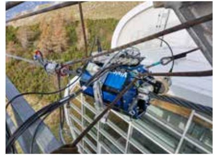
*3D rope measuring equipment assess rope quality from all sides*
