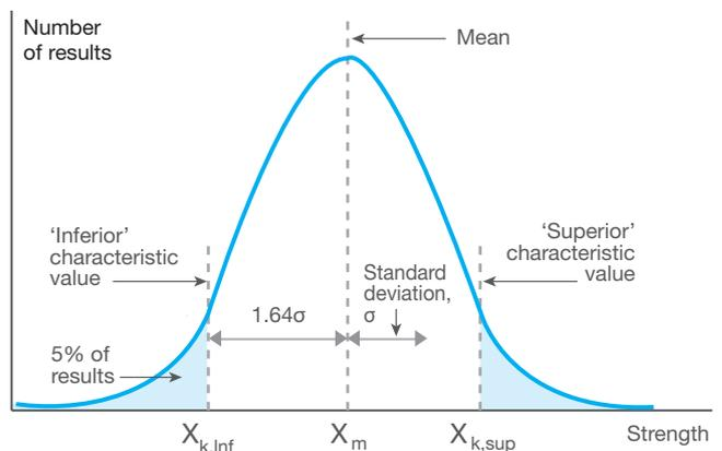
Fig. 6. Varying results possible from a set of identical samples.
