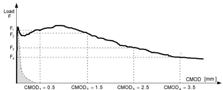
Fig. 3. Typical "force/crack width" trend.
