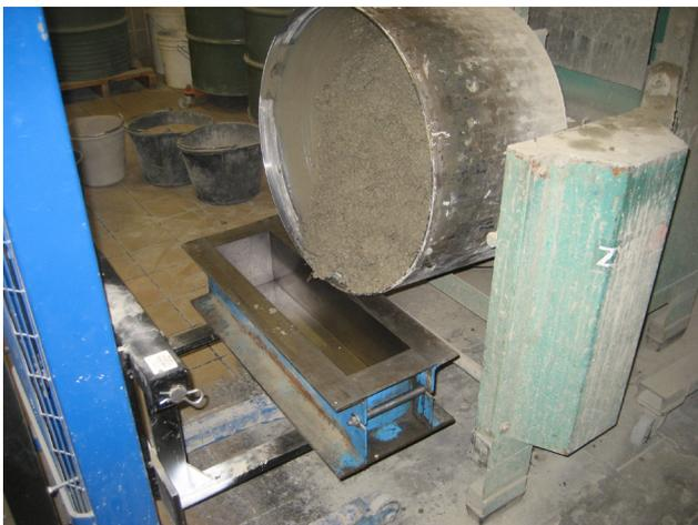
Filling the mould of an EN14651 beam
