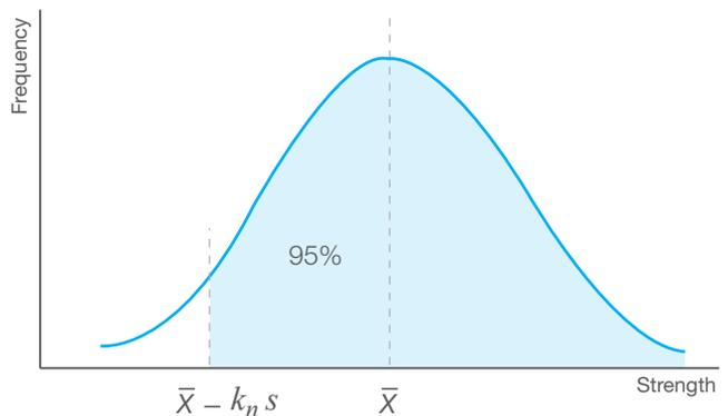
Fig. 5. Varying results possible from a set of identical samples.
