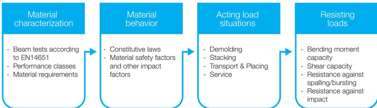
Fig. 1. Summary of a typical design process of FRC for precast segments.
