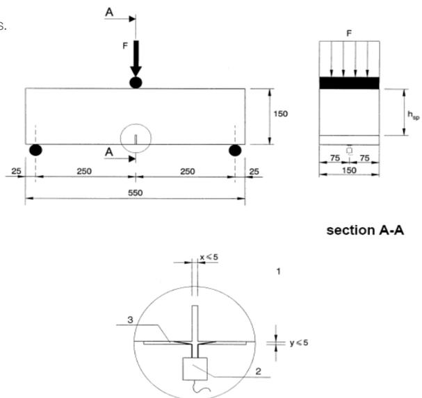
Fig. 2. EN 14651 test set up and geometry
