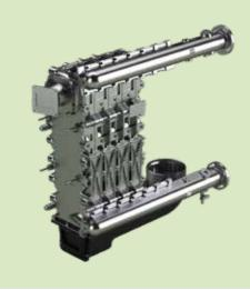
Aluflow® is a highly efficient commercial aluminum condensing heat exchanger with revolutionary hydraulic properties. The heat exchangers have a fully water cooled combustion chamber and requires no ceramic insulation. The high thermal conductivity
