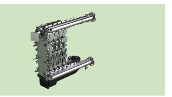
Aluflow® is a highly efficient commercial aluminum condensing heat exchanger with revolutionary hydraulic properties, 30mbar at full load with delta T 20°C. The heat exchangers have a fully water cooled combustion chamber and requires no ceramic insulation. The high thermal conductivity
