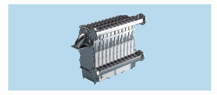
Alucom® aluminum condensing heat exchangers only need one cylindrical burner and one fan. The heat exchangers have a fully water cooled combustion chamber and require no ceramic insulation. The high thermal conductivity of the sectional casting
