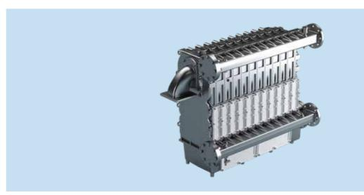
Alucom® aluminum condensing heat exchangers only need one cylindrical burner and one fan. The heat exchangers have a fully water cooled combustion chamber and require no ceramic insulation. The
