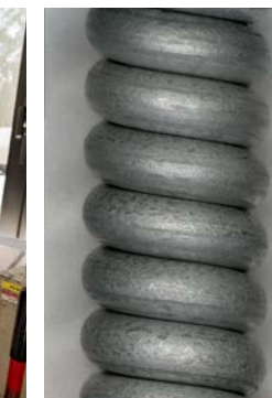
Bezinal® wires 80x magnifying ratio
