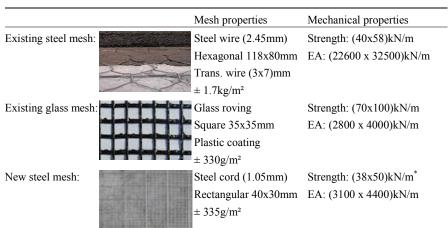
Table 1 Properties of metal and non-metal geotextiles used as anti-cracking interlayer
