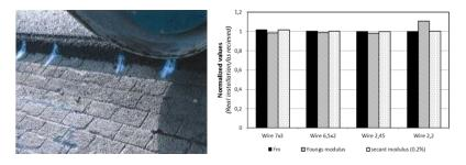
Fig. 2 Left: white paint indicates steel pieces installed under 4cm of asphalt; Right: normalized values for Fm, Youngs modulus and secant modulus at 0.2% from different steel half product
