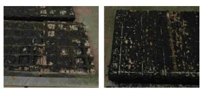
Figure 6: Left: Glass grid after being tested in horizontal plate test; the glass can be peeled off completely. Right: Steel cords anchored into the asphalt overlay.
