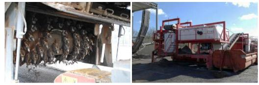
Figure 4: Left: Milling drum after grinding 100 m<sup>2</sup> asphalt reinforced with new steel grid. Right: Traditional breaking installation for asphalt foreseen with magnets.
