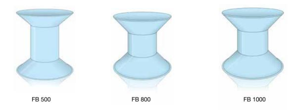
The spools have conical flanges. This reduces the angle by which the wire is paid off. This positioning of the spool puts less tension on the wire, allowing higher production speeds. To enable fault-free unwinding, the wires lay on the spools in a tapered fashion.
