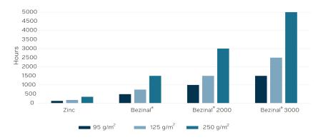
The salt spray method exposes various specimen, inside a cabinet, to a continuous spray of 5 % NaCl at a temperature of 35°C and relative humidity of 98%. The test measures the quality and performance consistency of metallic coatings. Salt spray testing is done accoording ISO 9227 and ASTM B117.
